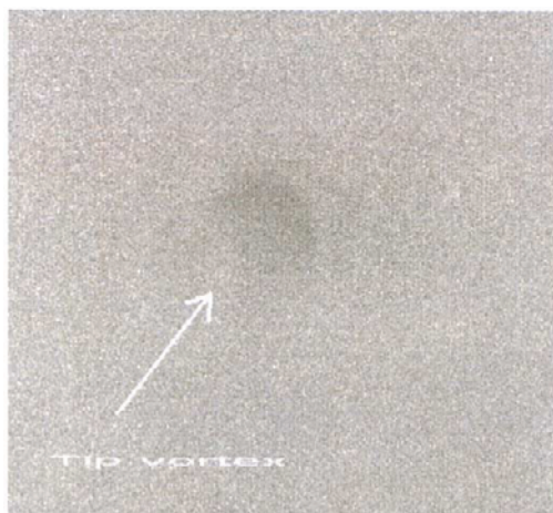
Fig. 2. Typical PIV recording of a propeller tip vortex ( 20 \times 20 \text{ cm}^2 ).
